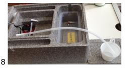
8. When you're finish, take off the used vessel and put the longer silicone tube to a connector and start the pump again to drain the remaining water into an external container. **Keep all power parts always dry !** Leave the box open for drying. When dry, put all material back to the box, close the lid and pull over the blue cover to store it until the next use/exercise
