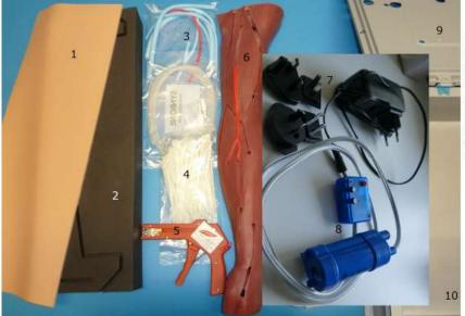
Box content: 1 skin with markings 2 black wedge to place the box 3 2 arteries & 5 veins 4 cable ties 5 cable tie applier 6 silicone arm 7 power supply with 5 connectors 8 pump with control unit 9 box cover 10 box body
